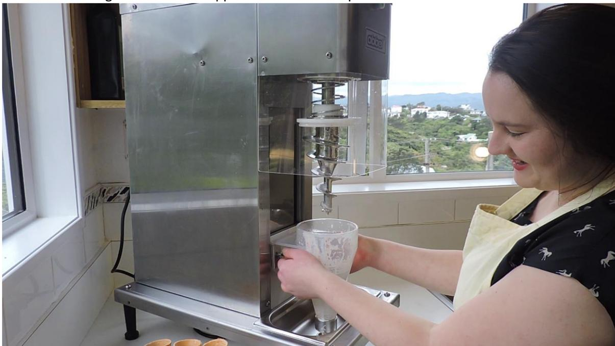
3. Wiggle the hopper off the machine (this can take a little force as there's a silicone seal in the middle that has to slide off).
