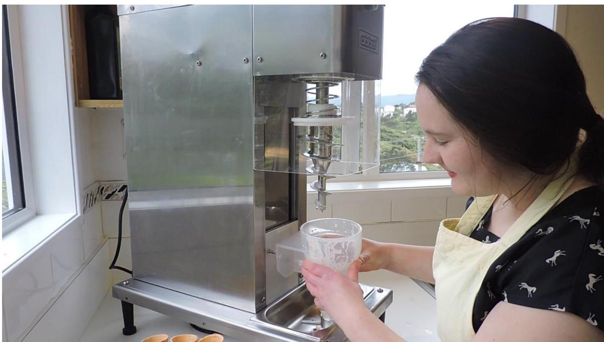
4. Remove the plastic shield. It sits on 4 little posts. Press the sides inwards so that they slide off their posts, then gently rotate it off the front posts.
